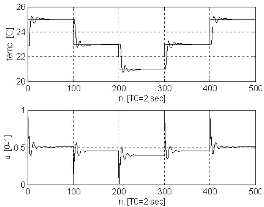
**Figure 4.** The performance of the optimal PID controller
