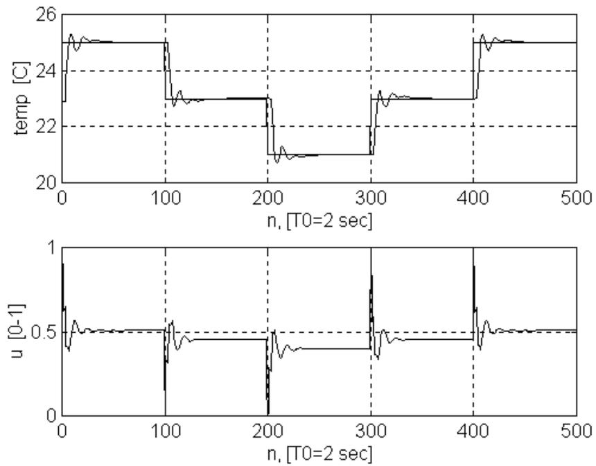
**Figure 7.** The performance of the optimised PID controller (simulation, Perf=114.7)
