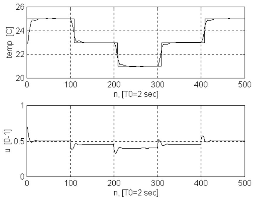
**Figure 8.** The performance of the HFCM based controller
