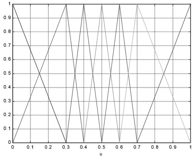
**Figure 4** Membership functions on the control signal,  $u_s$
