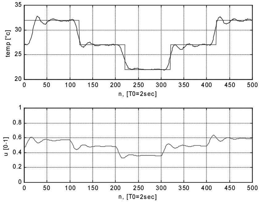
**Figure 11** Real time control performance by using the HFCM based controller
