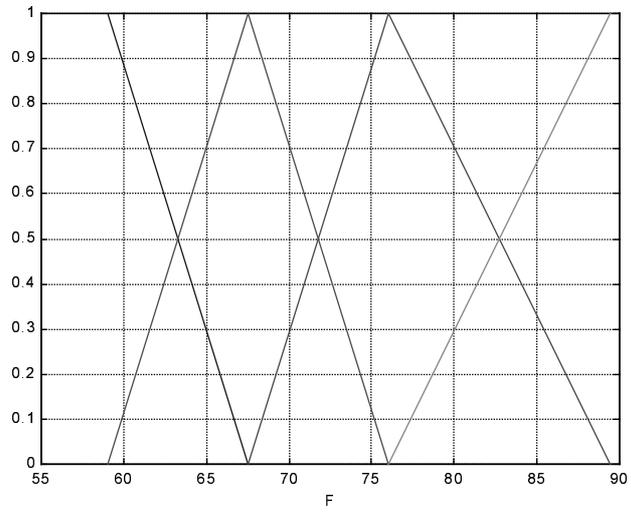
**Figure 3** Membership functions on the input flow rate,  $F$
