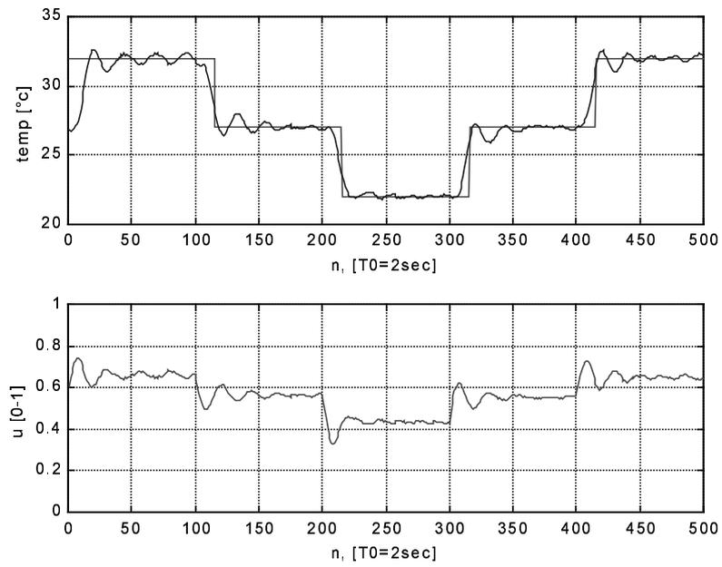
**Figure 10** Real time control performance by using the HFCM based controller
