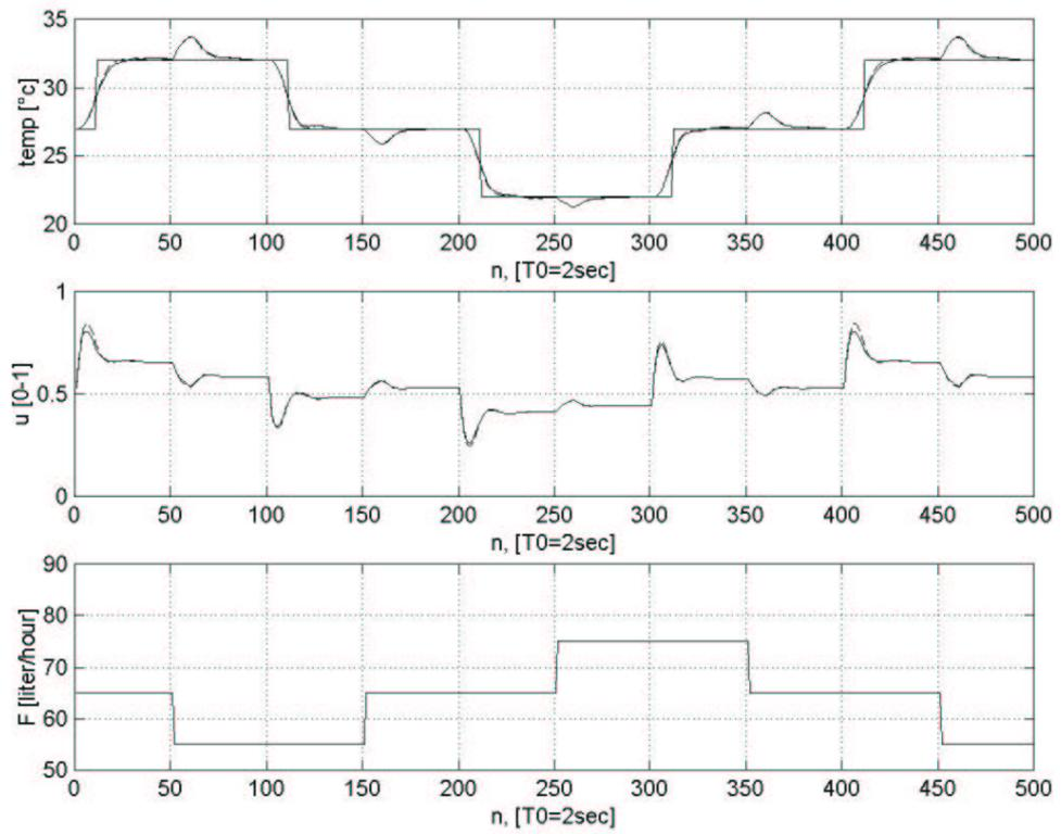
**Figure 9** Comparison of the hybrid fuzzy model based controller, ‘-’ and an *a priori* model based gain-scheduled DMC controller, ‘--’
