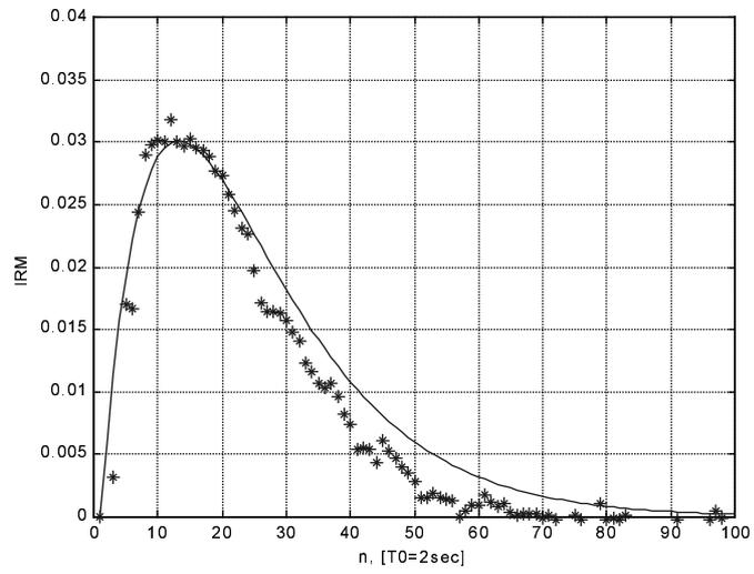
**Figure 6** Measured and fitted impulse response model at given flow rate (\* measured, - fitted)
