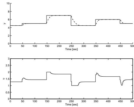
**Figure 4.** Control performance of the globally identified, Lyapunov-linearization based MPC.
